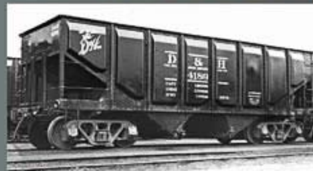
Figure 1: The Delaware & Hudson got a thousand USRA twin hoppers immediately following World War I and numbered them D&H 3201-4200. In the 1930s, more than three hundred of them were rebuilt with panel steel sides. Only a month after being rebuilt at the Oneonta, NY shops, D&H 4180 was at Binghamton, NY in September, 1936. Panel sides increased its cubic capacity from 1880 cubic feet to 1940 cubic feet. Note its original USRA Andrews trucks. -Keith Sirman collection
